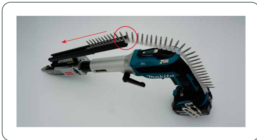
Abbildung/Illustration 10 • Inserting screw autofeed – Step 1
