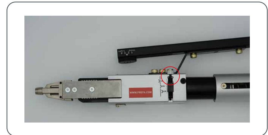
Abbildung/Illustration 9 • Adjusting screw-in depth
